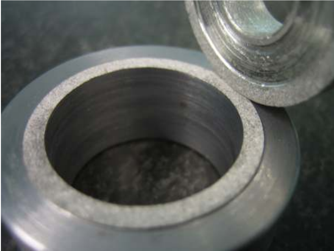
Figure 1: Test piece showing fractured area
